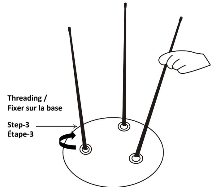
**Warning :** Do not over-tighten. Over-tightening can cause threading to slip.
